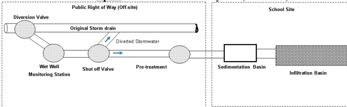
Error! Reference source not found.2 is the plan view of the same concept. Both figures highlight the potential components that can be included in such an effort. It is assumed that the stormwater is flowing down the side of the street in the curb and gutter, and additional maintenance holes are strategically placed to divert, monitor and pre-treat the stormwater.
